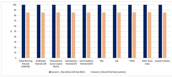
Comparison between the results of Scenario 1- Yacht without submerged wing (BAU) and Yacht with Hull Vane submerged wing (Innovative Solution). The results are expressed in percentage.
