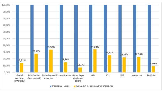
Comparison between the results of the Scenario 1- Yacht with neoprene fender cover (BAU) and Scenario 2- Yacht with bioprene Fendaskin (Innovative Solution). The results are expressed in percentage
