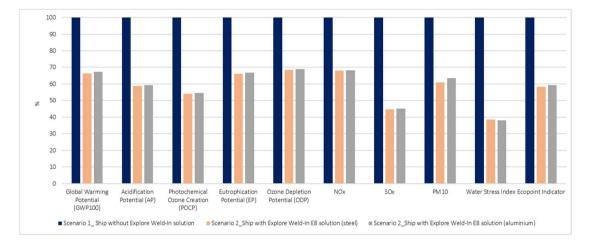
Comparison of environmental impacts between the results of Scenario 1- Yacht without Explore Weld-In solution (BAU) and Yacht with Explore Weld-In E8 solution. The results are expressed in percentage.
