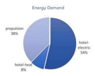
From the hotel load over 50% is used by the HVAC system. Several options are available to reduce this load.
