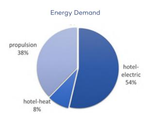
From the hotel load over 50% is used by the HVAC system. Several options are available to reduce this load.
